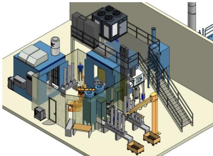
Exhibition 2: Automated thermal coating and blasting machine as an example of automated machines
